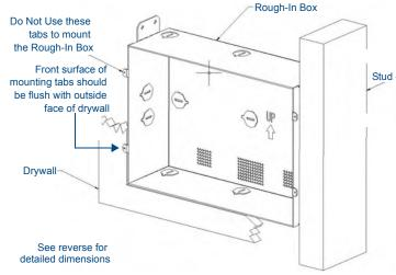
FIG. 1 CB-TP10 - Drywall Installation
